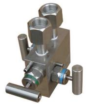
The 3VD-35 valve block is used to shut off the connection to the process and to equalize the pressure between the two inputs of the differential pressure gauge before the actual measurement.
