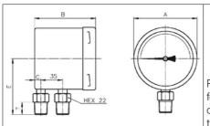
PDR02...K: for pipe mounting, connection at bottom
