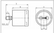
PDR02...M: for pipe mounting, connection at back
