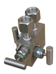
The 3VD-35 valve block is used to shut off the connection to the process and to equalize the pressure between the two inputs of the differential pressure gauge before the actual measurement.
