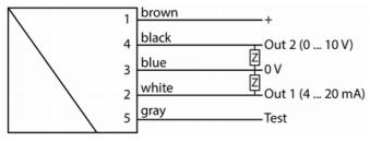
Attention: Pin 5 must not be electrically connected! We strongly recommend use of a four core cable.
