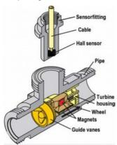
These hit the rotor from four directions and cause it to turn. Due to the uniform load on the bearing from four sides, most of the forces are balanced and wear is reduced to a minimum. The extremely hard bearing materials, sapphire and tungsten carbide, also guarantee an exceptionally long service life.
