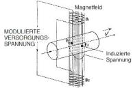
induces an electrical voltage in the liquid. This voltage is picked up by two electrodes inserted in the measuring tube and further processed by the downstream electronics. The level of the voltage is proportional to the flow velocity.
