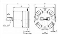
PDR04...N for panel mounting, with three-hole front ring, connection at back
