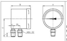
PDR02...K: for pipe mounting, connection at bottom
