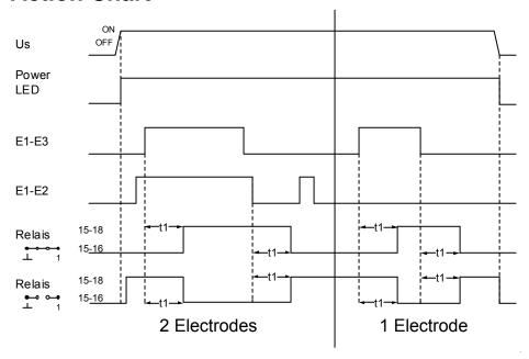
t1 = adjusted switching-delay LED Relay on = relay
