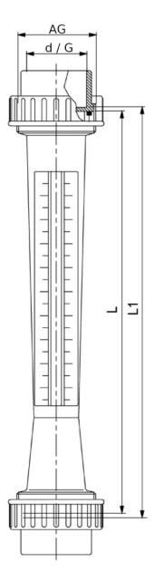
PVDF measuring tubes have different dimensions L and L1.
