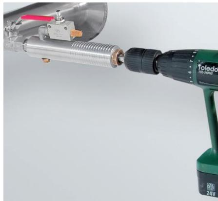
In case the system could not be shut down, means to be set depressurized, there could be used the spot drilling collar (please request) to drill through the ball valve.
