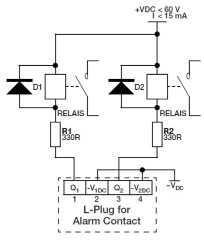
Variant 2: elctrical connection of contact outputs: I > 15 mA
