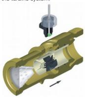
One part of the liquid flow causes the turbine to rotate, while the other part flows unhindered through the annular gap. The rotor speed is now converted into an electrical pulse signal (frequency). High-quality sapphire bearings and low speeds ensure that the turbine has an exceptionally long service life.
